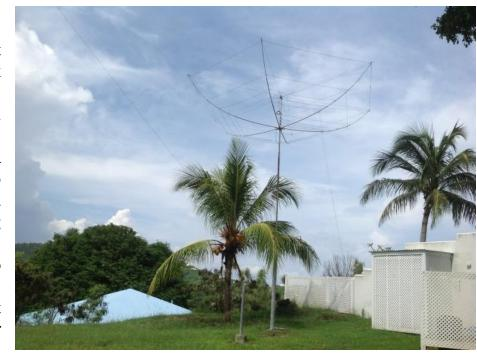
Average temp during our stay was 85deg...every day, and just a 10deg cooler at night. Above pix is of the hexx-beam. It has 5 bands in one antenna (20M thru 10M with 17m and 12m, too).
