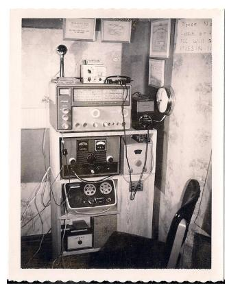
In 1962 I apparently abandoned the Morse code mode of communication as I restructured my station but without a comfortable place for the Morse code keyer (the microphone is prominent with the J-38 keyer relegated to the top of the VFO).
